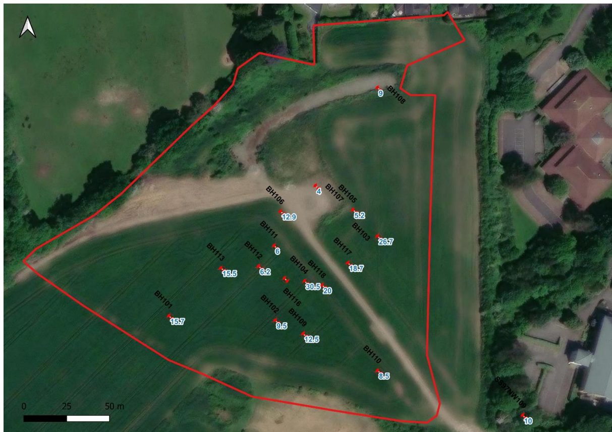
Figure 5.2 Summary of Depth to Bedrock during Rotary Drilling
